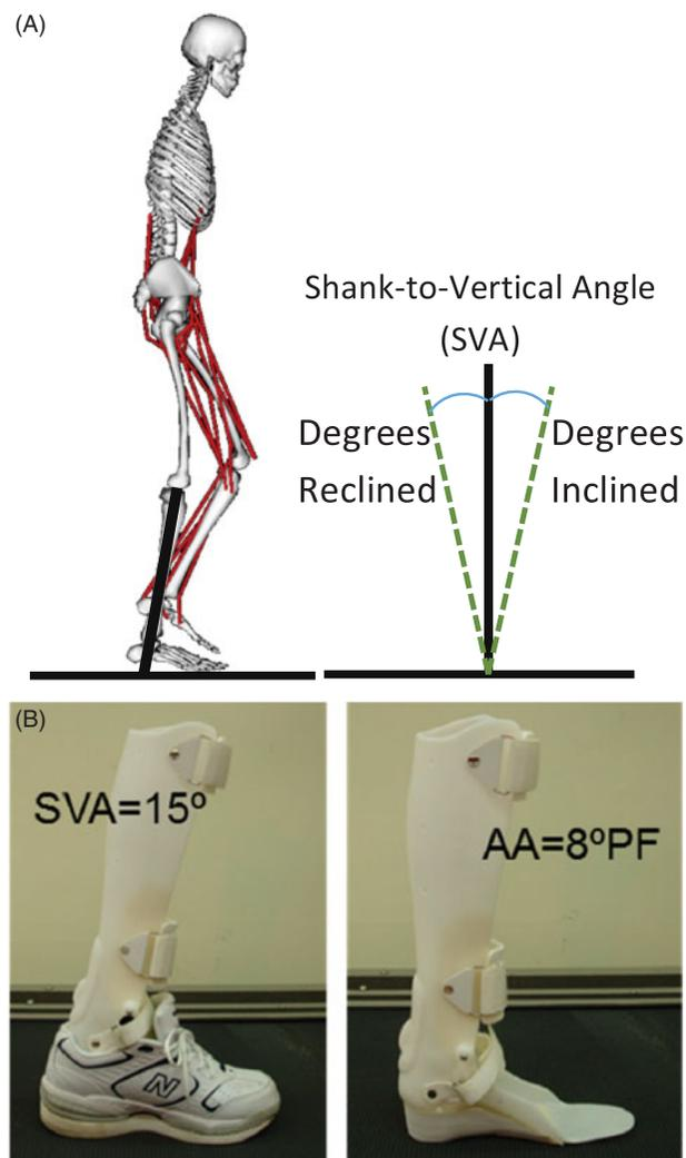
Figure 1. (A) Shank-to-vertical angle (SVA) is defined as being either reclined or inclined. During normal walking, the SVA at midstance is 10° inclined. (B) Alignment of the AFO-FC showing ankle angle (AA) set at 8° plantar flexion and SVA of 15° inclination when the orthosis is placed inside a modified shoe.
